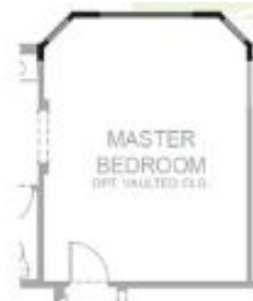
Bay Window at Master Bedroom
